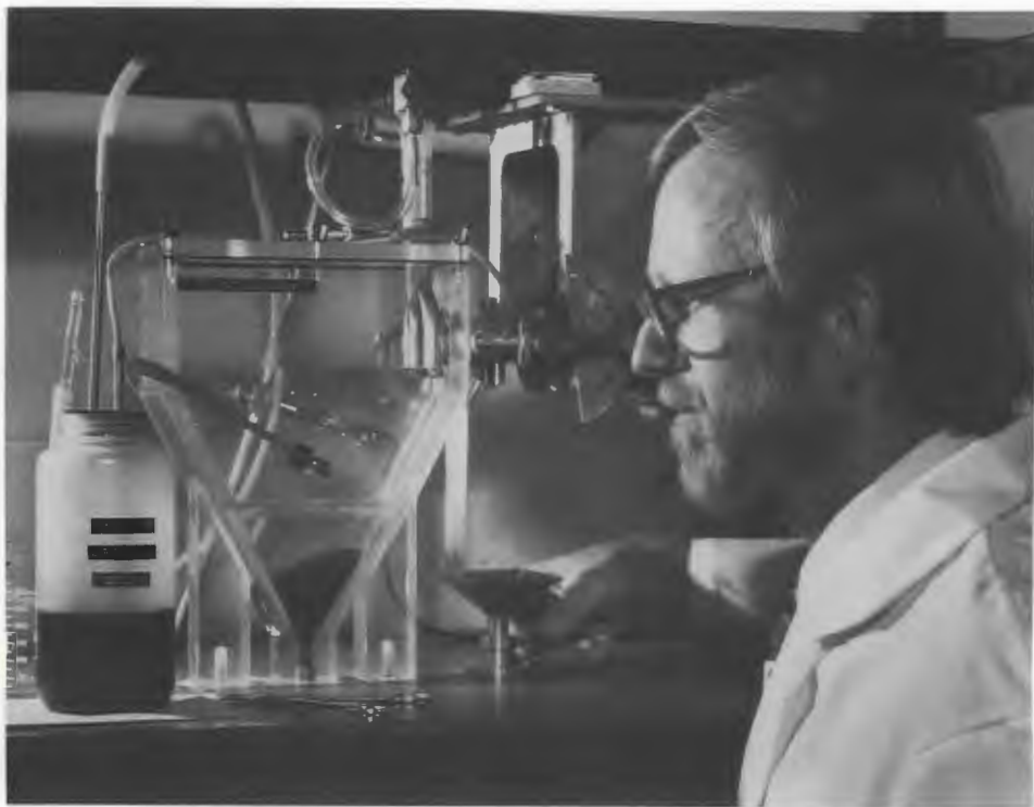
Helmut Ringel, guest scientist from Germany last year, observes the formation of uniform beads of nuclear fuel produced by the Gel-Sphere-Pac process developed here.
