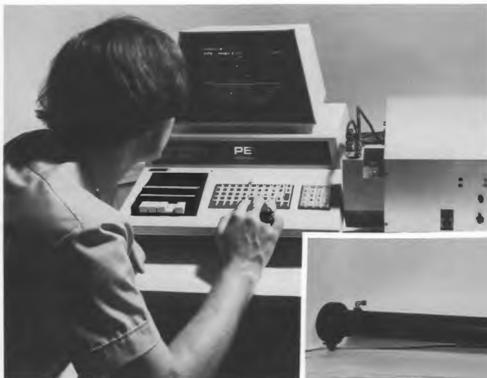
Working at the personal computer interfaced with the derivative ultraviolet-absorption spectrometer (DUVAS), Alan Hawthorne determines the amount of a specific polynuclear aromatic compound present in an air sample. Pictured in the inset is the DUVAS with air sampling tube. The instrument can detect hazardous compounds in coal-derived gases and tars.
