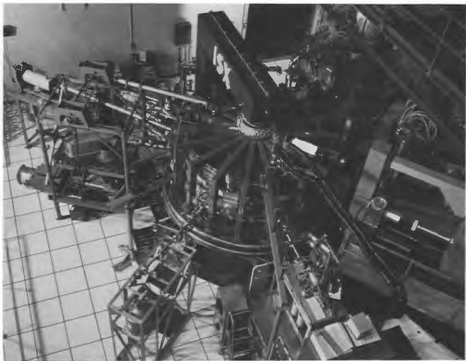
A pellet-refueling technique for fusion reactors was demonstrated with ISX-A. Refueling is essential for maintaining or increasing plasma density.
