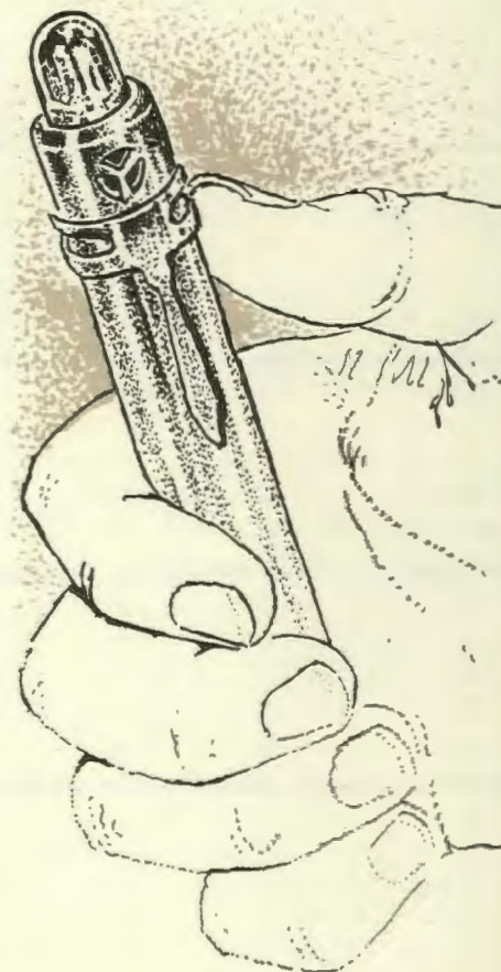
The personal radiation monitor (PRM) chirps or screams in response to rising levels of gamma radiation.
