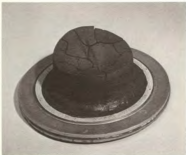
This is a coal precoat deposited on a 3-in. filter screen showing the accumulation of the solids on the precoat surface.
