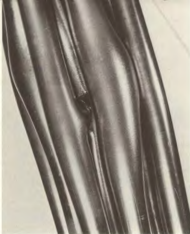
The region of maximum swelling in a 13-rod bundle tested in argon is shown here. Two ruptures are visible in the Zircaloy fuel cladding. These tests, run in 1971 by Phil Rittenhouse and Ralph Waddell, show dramatically that, under certain test conditions, severe coolant blockages can occur.
