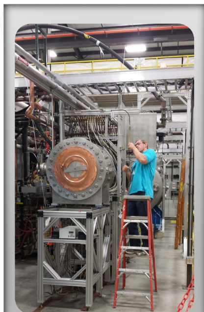
Installing a 4 mm microwave interferometer on Proto-MPEX to measure plasma density
