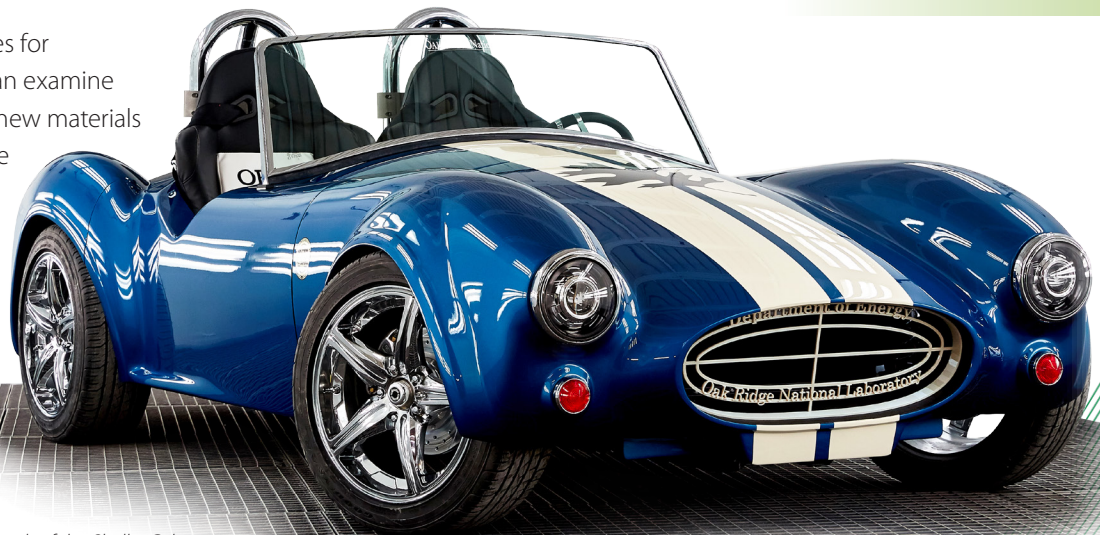
The frame and body panels of this Shelby Cobra replica were 3D-printed at ORNL.
