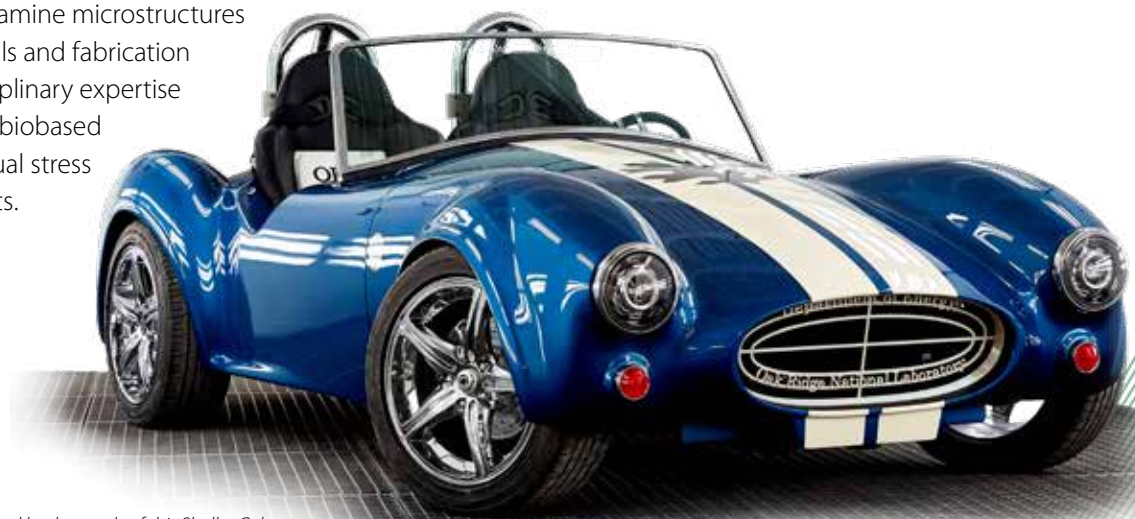
The frame and body panels of this Shelby Cobra replica were 3D printed at ORNL.
