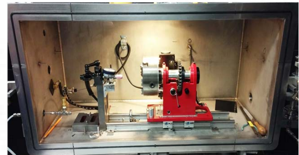
The AXEL vacuum chamber: CAD model (top) and internal configuration of the welding equipment (bottom).
