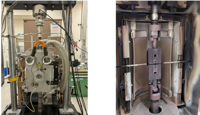
**Figure 7.** LEFT: Instron frame with MRF furnace for elevated temperature tensile testing; RIGHT: The TZM tensile fixture placed at the center of furnace hot zone.
