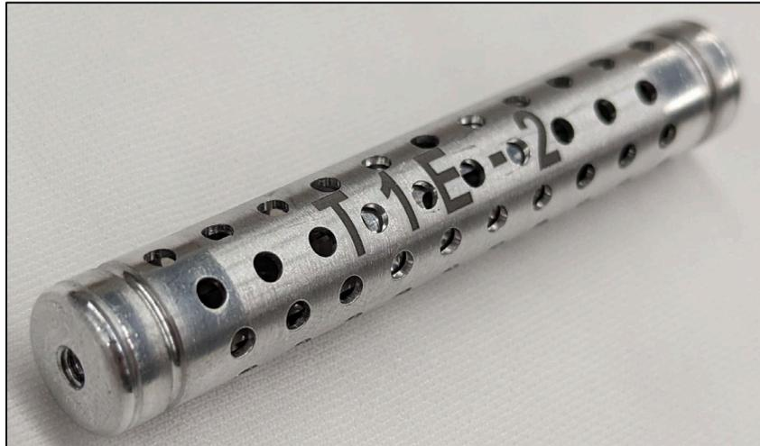
**Figure 6.** Final T1E-2 capsule prior to HFIR insertion.
