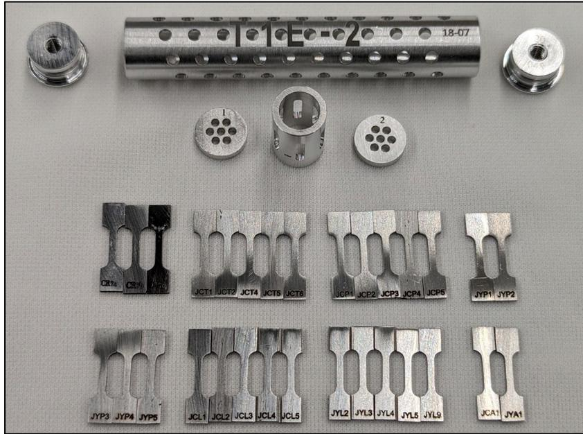
**Figure 5.** The T1E-2 parts laid on lint free towel prior to assembly.
