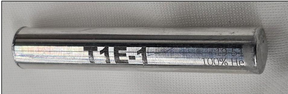
Figure 3. Final T1E-1 capsule prior to HFIR insertion.
