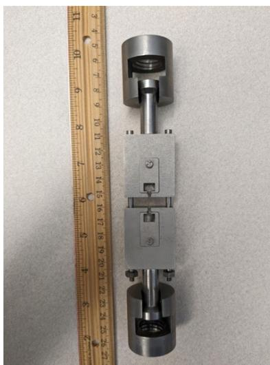
**Figure 4.** Shoulder-loaded TZM tensile fixture.
