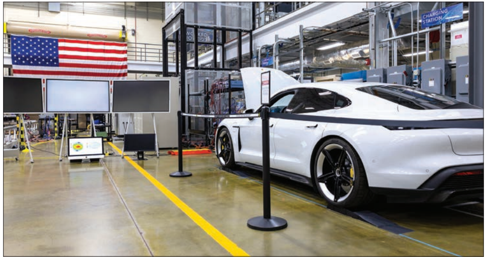
ORNL researchers collaborated with Volkswagen Group of America to demonstrate wireless 270-kW power transfer to a Porsche Taycan. Image credit: Carlos Jones, ORNL
