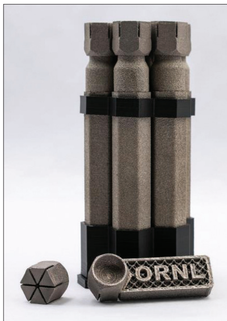
ORNL researchers used electron-beam additive manufacturing to 3D-print the first complex, defect-free tungsten parts with complex geometries. Image credit: Michaela Bluedorn, ORNL
