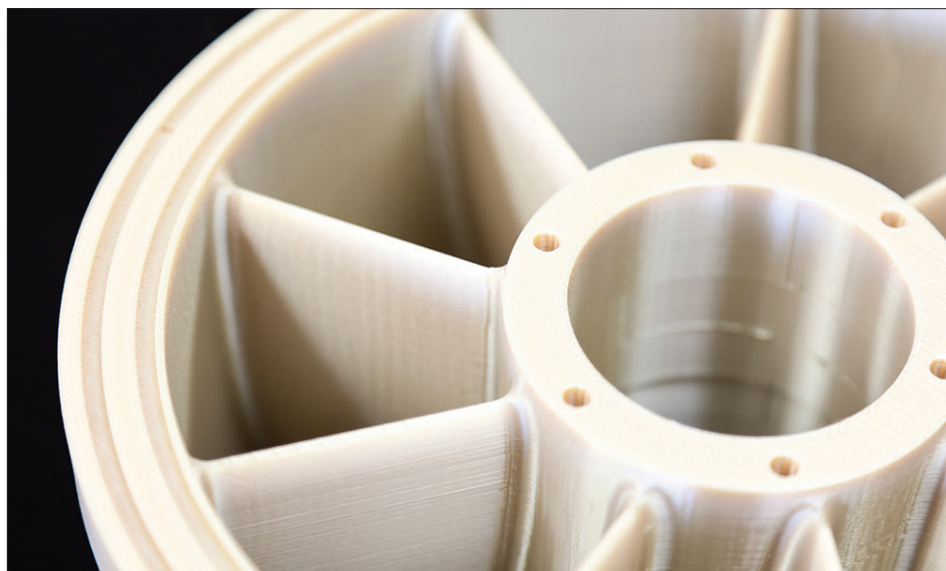
This newly manufactured fixed guide vane of a hydropower turbine system was printed at the DOE Manufacturing Demonstration Facility at ORNL. Image credit: Genevieve Martin, ORNL
