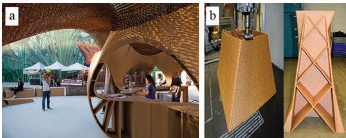
Figure 1. (a) 30-meter-long bamboo-PLA installation at Design Miami 2016 printed at ORNL's Manufacturing Demonstration Facility; (b) large-scale 3D printing process using poplar / PLA composite (left photo), and a completed 3D printed podium base (right photo: back of podium base). [Credits: (a) ORNL internal images, (b) Reprinted [adapted] with permission from Zhao et al. [6] Copyright 2019, American Chemical Society].
