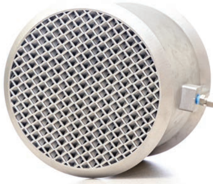
Figure 1. Additively manufactured PIPE for increasing CO 2 capture efficiency in solvent-based systems via integration of heat exchange functionality [Photo credit: C. Jones, ORNL].
