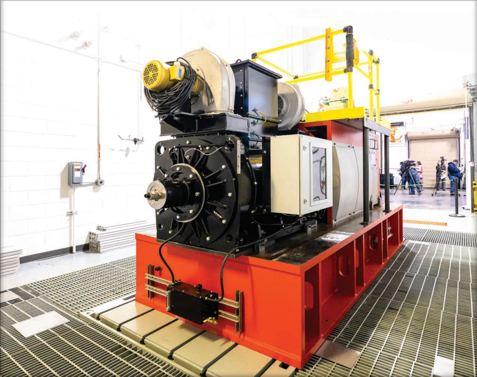
A single-cylinder locomotive engine was installed at DOE's National Transportation Research Center at ORNL to study the integration of hydrogen as an alternative fuel source for diesel-powered railways. Image credit: Carlos Jones, ORNL
