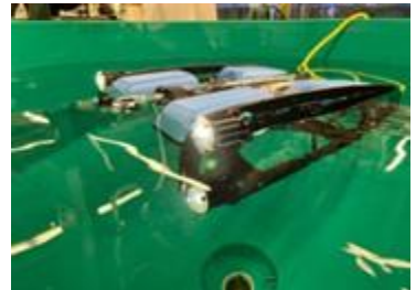
ORNL's submersible ROV undergoes leak testing prior to field deployment.
