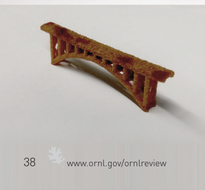
A novel polymer developed at ORNL strengthens sand for additive manufacturing applications. A 6.5 centimeter 3D-printed sand bridge, shown here, held 300 times its own weight. Image credit: Dustin Gilmer, University of Tennessee, Knoxville
