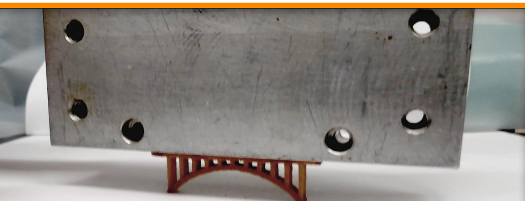
A novel polymer developed at ORNL strengthens sand for additive manufacturing applications. A 6.5 centimeter 3D-printed sand bridge, shown here, held 300 times its own weight. Image credit: Dustin Gilmer, University of Tennessee, Knoxville
