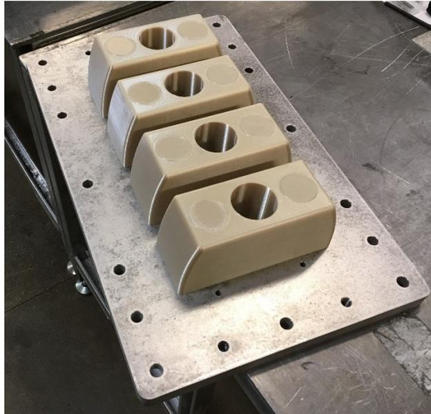
**Figure 3: Fabricated Top Mold**
