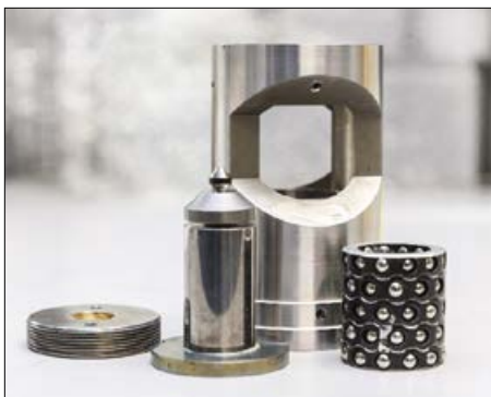
The diamond anvil pressure cell uses two gem-quality synthetic opposing diamonds to exert extreme pressures on materials, providing fundamental insights into materials that only neutrons can reveal. Image credit: Genevieve Martin, ORNL
