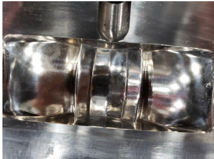
Figure 7. Mold surface after polishing.
