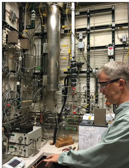
A pilot reactor, developed by Vertimass and located at TechnipFMC, can scale up the process that converts ethanol into fuels suitable for aviation, shipping and other heavy-duty applications. Credit: TechnipFMC
