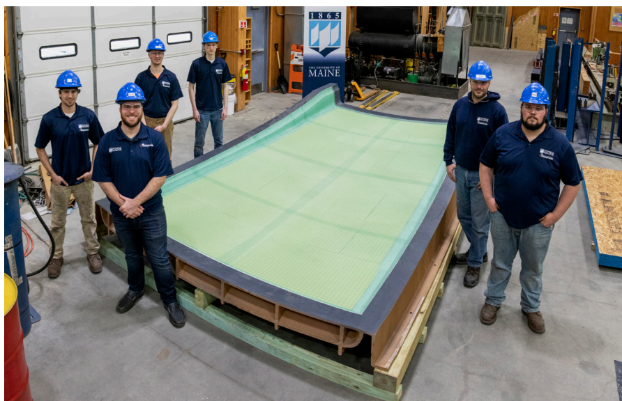
The University of Maine and ORNL collaborated on this large-scale boat mold printed using biobased materials.
