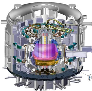
Fusion thermal power has already been demonstrated in tokamaks; however, a sustained burning plasma has yet to be created. The ITER tokamak is designed to achieve an industrial-scale burning plasma producing 500 megawatts of fusion thermal power. ITER's plasma volume is more than eight times greater than that of the largest existing tokamak.
