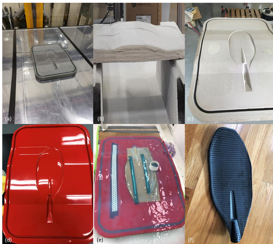
Fig. 3. (a) PRD-1520 printed mold, (b) High build coating and machining, (c) Finished mold for gel coat, (d) Gel coated and polished mold, (e) Sprayed silicon bag, (f) Carbon fiber kayak paddle
