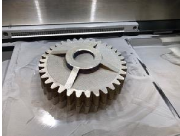
Figure 3 shows the prototype Ferrium C64® gear with mesh in the hub with solid band and teeth
