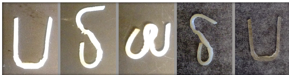
A new plastic developed by ORNL and Washington State University transforms from its original shape (left) through a series of temporary shapes and returns to its initial form. The shape-shifting process is controlled through changes in temperature. Image credit: Washington State University
