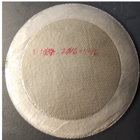
Figure 10: Plate with high resistance to gas flow.
