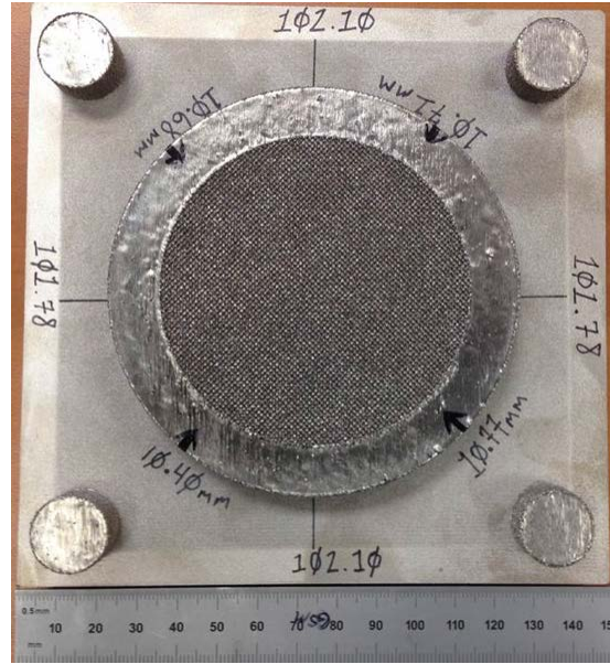
Figure 3: Example top view of porous disc fabricated in this work through electron beam melting.
