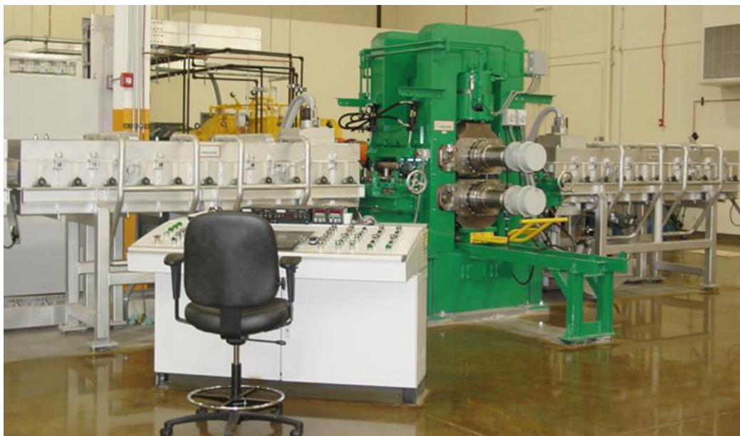
Figure 2. MDF isothermal shear rolling mill.
