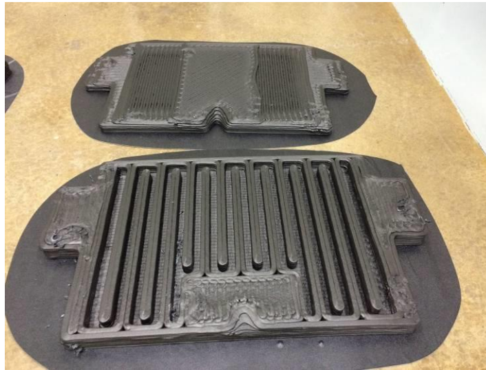
Fig 4. Printed Freezer Door Tool with Integrated Fluid Passageways
