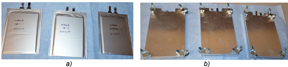
Figure 1. NMC/CB and NMC/graphene pouch cells a) individual pouch cell and b) test units
