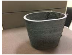
(a) As-printed BAAM magnet
