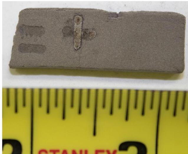
**Figure 21. Cross shape built vertical line first. The horizontal line didn't fully sinter due to interference from the vertical line.**
