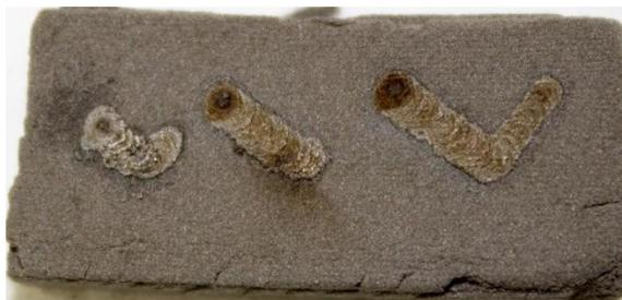
**Figure 22. Zig-zag shape built with an upward move direction in the vertical sections. The vertical sections didn't fully sinter due to interference from previously sintered spots.**
