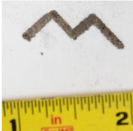
**Figure 16. Zig-zag shape created by chaining sintered dots.**
