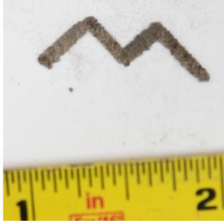
**Figure 23. Zig-zag shape built with a downward move direction in the vertical sections.**
