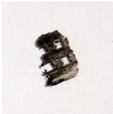
**Figure 33. Sintered part showing fine detail captured where there was a lack of bound powder.**
