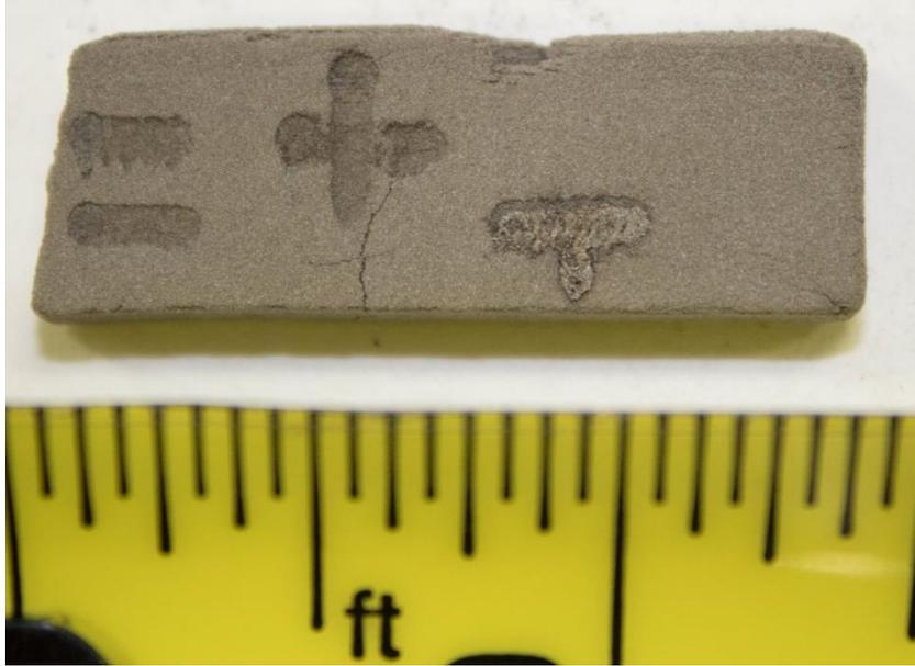
**Figure 20. Cross shape built horizontal line first. The upper half of the vertical line didn't sinter due to interference from the horizontal line.**
