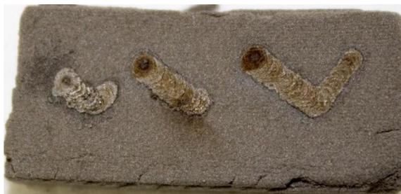
**Figure 22. Zig-zag shape built with an upward move direction in the vertical sections. The vertical sections didn't fully sinter due to interference from previously sintered spots.**
