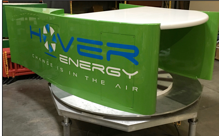
Fig. 2. HE2.0 unit without rotor blades installed. Green and white diverters are hand layup vacuum infused molding of glass and carbon fibers.
