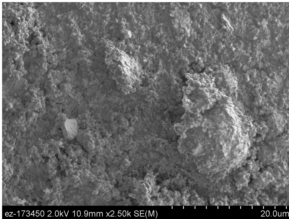
Fig. 1. SEM of "SG" \text{Al}_2\text{O}_3 powder (agglomerated fine particles).
