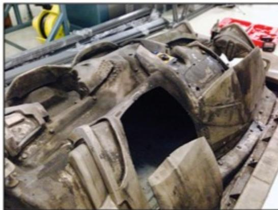
**Fig. 2. Picture of nickel tooling with a segment removed.**
