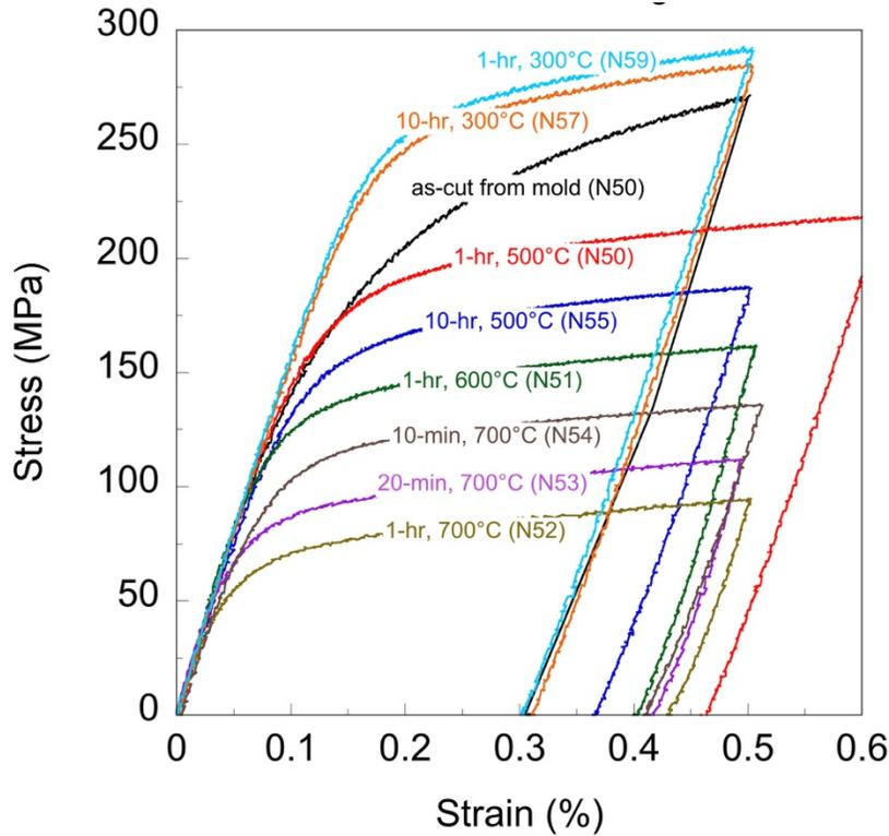
**Fig. 9. Tensile stress-strain response for different specimens removed from the mold to illustrate the effect of both temperature and time of thermal annealing to remove strain hardening from the nickel tooling.**
