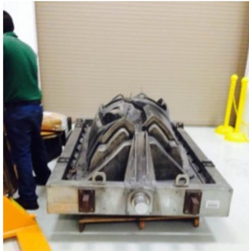
**Fig. 1. Picture of nickel tooling received from Faurecia for this investigation. Note person on the left for scale.**
