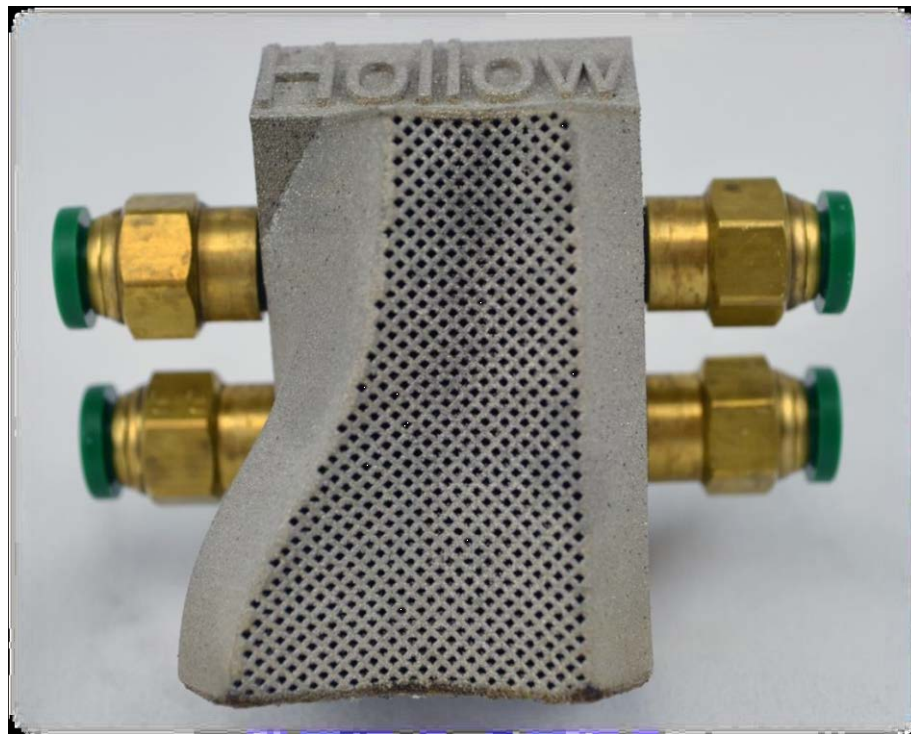
Fig. 4. Redesigned electrode fin.
