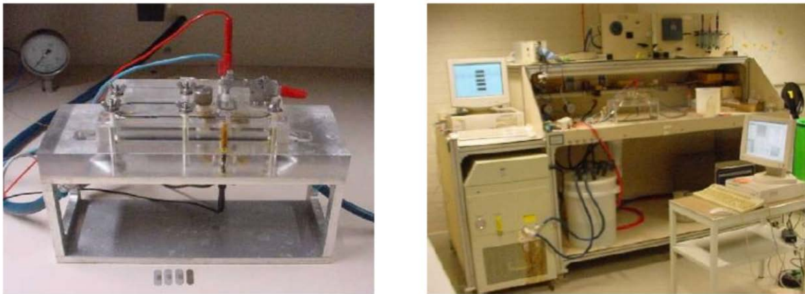
Fig 1. Flow Channel Cell (FCC) and related equipment.
