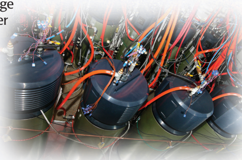
Heat pump water heater accelerated durability testing
