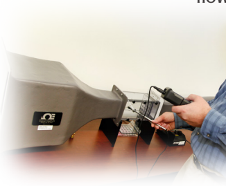
Bench top wind tunnel
