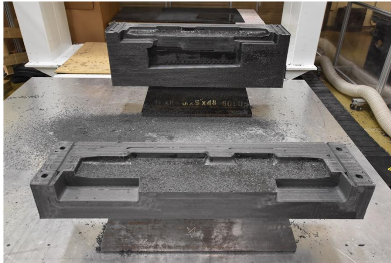
Fig. 4. The top and bottom sections of the casting pattern with epoxy applied to them to fill voids that occur during the printing process and are revealed during the machining process.
