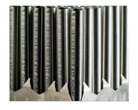
New **accident tolerant fuel (ATF) cladding**, conceived, developed, manufactured, and tested at ORNL, has been manufactured by Global Nuclear Fuels (GNF) into lead test assemblies, and shipped to Southern Nuclear Operating Company for trials in Edwin I Hatch plant. The FeCrAl cladding, called IronClad (see figure), will be the first developed through DOE's Enhanced ATF program to be installed in a commercial nuclear reactor. (February 2018)
