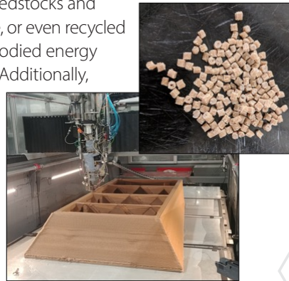
Bio-based feedstock Poly(lactic acid) (PLA)/wood fiber composite pellets (top) and utilization in Additive Manufacturing process (bottom)
