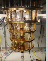
A dilution refrigerator run by the Quantum Information Science group. This refrigerator operates at a base temperature of roughly 10 mK and includes optical and scanning probe microscope heads for material and device characterization at low temperatures.
