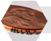
MiniFuel—a small-scale, ORNL-designed experiment—drastically decreases the size of fuel specimens and capsules irradiated in HFIR. The unique platform will allow for faster qualification of new nuclear fuels, providing economic benefits to nuclear power plant operators.
