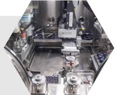
The Radiochemical Engineering Development Center is the largest hot cell facility at ORNL, with 15 hot cells that allow scientists to safely handle radioactive materials for processing, testing, recovery, and purification. The facility includes unique laboratory spaces to chemically process materials and pursue new isotope production techniques that reduce costs and improve outcomes.
