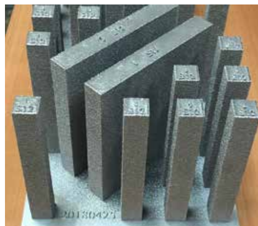
The Haynes 282 superalloy was fabricated into rods and plates for analysis of its suitability in advanced gas turbines.
