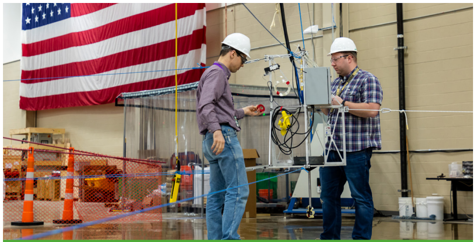
ORNL researchers with SkyBAAM, an additive manufacturing system used to 3D print the EMPOWER wall. Photo credit: Oak Ridge National Laboratory, US Dept. of Energy.
