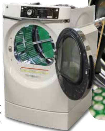
The energy efficient ultrasonic dryer developed at ORNL extracts moisture with high frequency vibrations.
