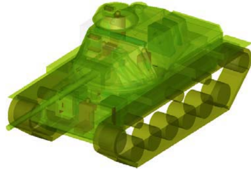
Fig. 3. MCNP/BRL-CAD models of simplified M60A1 tank geometry.
