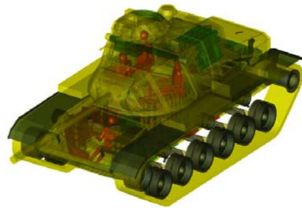
Fig. 1. A sample complicated geometric model prepared using BRL-CAD; M60A1 tank model with its crew.
