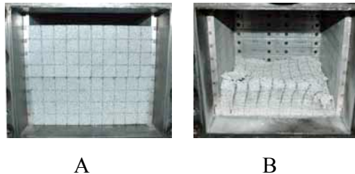
Figure 1. A) Image of the 40 PPI aluminum foam loaded in shock tube before test. B) Image of post shock compression of the aluminum foam.
