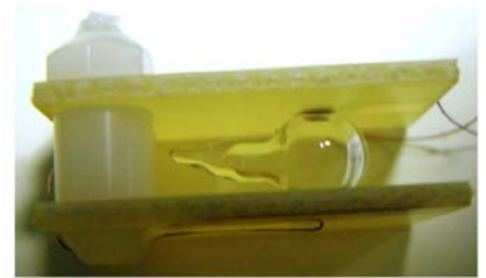
First generation gas-filled shell held between circuit boards.
