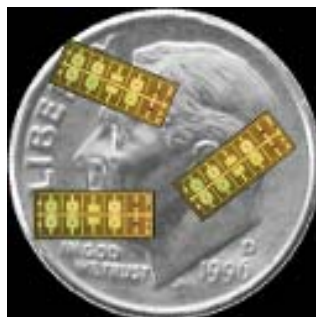
Fig. 2. MEMS sensor array building environment monitoring.
