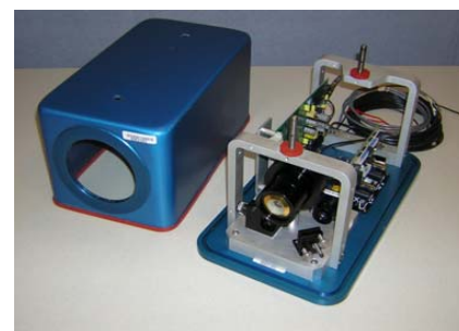
Fig. 3. Laser-based item monitoring system for high-value storage environments.
