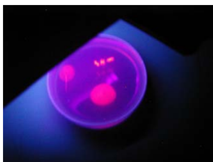
Fig. 1. Thermoluminescent nano-powders for harsh environment temperature sensing.
