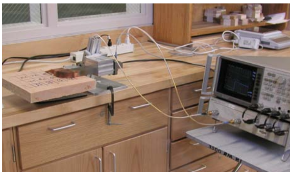
Microwave moisture measurement system for lumber drying.
