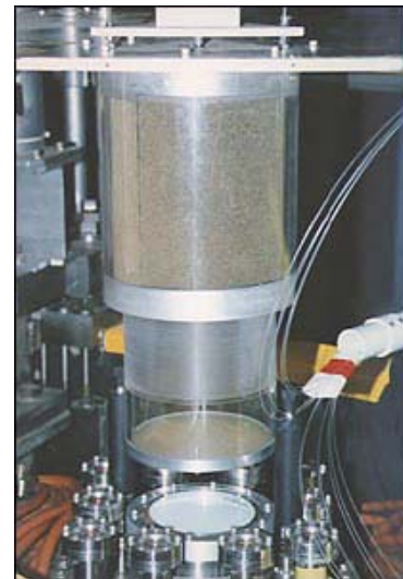
Millimeter-wave radiometer for measuring plasma electron temperature.
