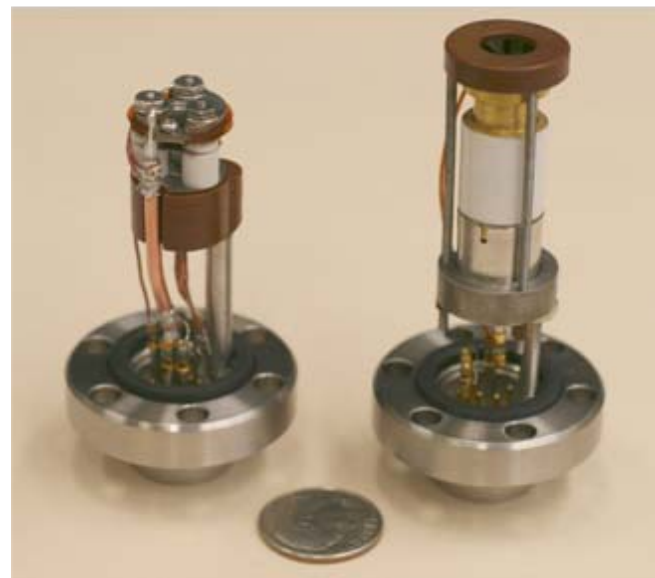
Mass analyzer components for the hand-portable mass spectrometer
