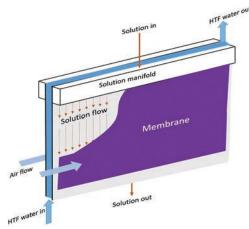
A new class of gas-fired heat pump water heater systems, based on a novel semiopen sorption concept, replaces the evaporator in a traditional closed sorption device with a permeable membrane that more efficiently absorbs and transfers heat for residential applications.
