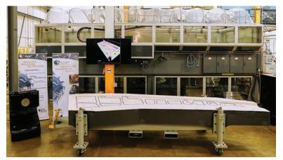
A 3-D-printed trim tool developed by ORNL and Boeing to be used in building Boeing's 777X passenger jet has received the title of largest solid 3D printed item by Guinness World Records. (Photo by Carlos Jones)
