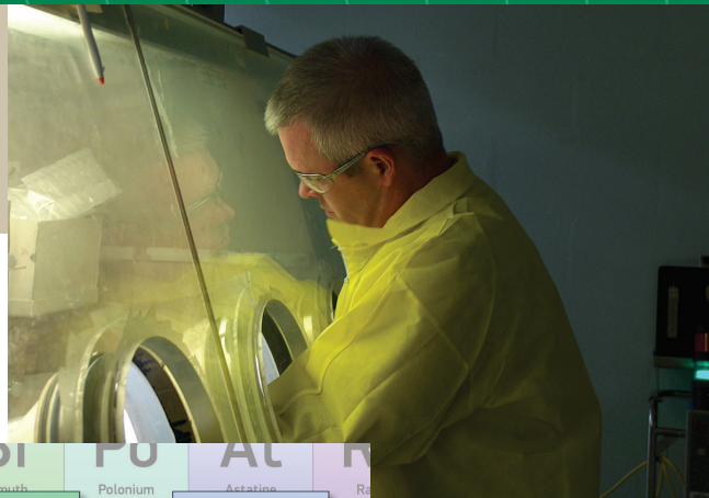
Frank Riley of ORNL’s Reactor and Nuclear Systems Division carefully prepares the berkelium-249 that would become element 117 material in a glove box at ORNL’s Radiochemical Engineering Development Center. (ORNL photo)
